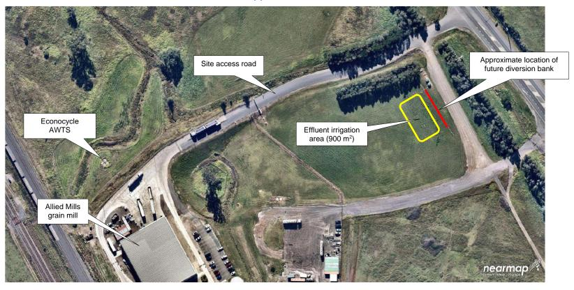
Figure 1: Wastewater irrigation area and location of diversion bank
